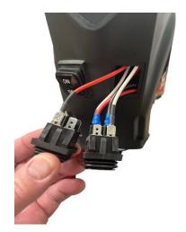
When all 6 terminals are replaced, gently push the new switch into the housing until it locks in place.
