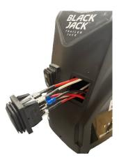
When the switch is out, use the flat blade screwdriver to remove one terminal at a time. Once the terminal is removed, place it in the same position on the new switch.
