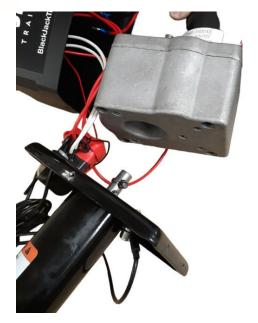
Step 4 Using a number 5 Allen key, unscrew the 4 bolts on the underside of the gear box. These bolts hold the motor and gear box together.
