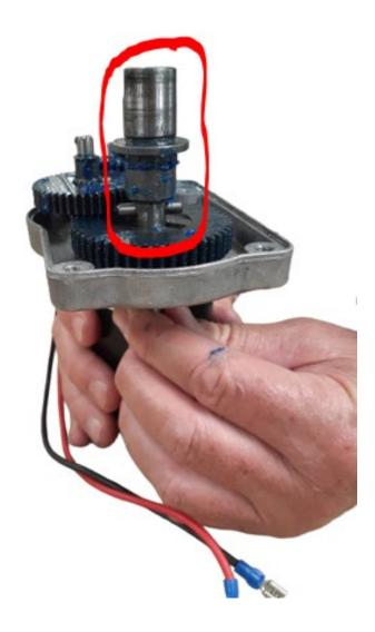
Remove all broken pieces as you don't want any metal fragments floating inside the gear box.
