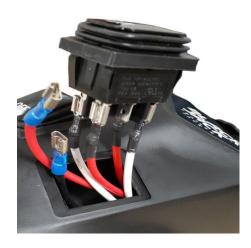
When the switch is out, carefully remove the 2 middle wires. There are 3 rows of 2 wires, remove the middle 2, these are the positive and negative wires to the motor. By disconnecting them now, you will have free access to the motor and gearbox later.
