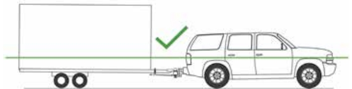
GOOD: Trailer is level, rear of tow vehicle is a little lower than front
