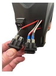
When all 6 terminals are replaced, gently push the new switch into the housing until it locks in place.
