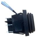
To remove the switch, take a flat blade screwdriver and gently pry the switch out at the top and the bottom. Take it slowly and the switch will gradually come out.
