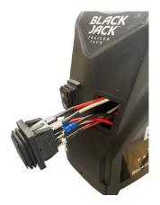
When the switch is out, use the flat blade screwdriver to remove one terminal at a time. Once the terminal is removed, place it in the same position on the new switch.
