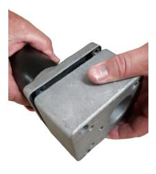
Use a bit of force to separate the gear box from the motor. It is a tight seal, so a bit of force is necessary. The use of a small hammer to tap on the main shaft will help separate the motor and gear box. The main shaft is in the circular recess, give it a gentle tap.
